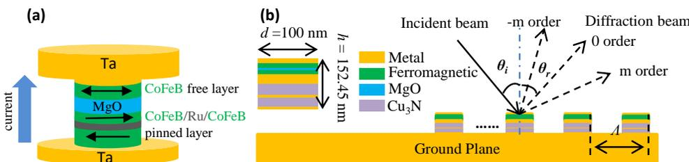
Fig. 1. (a) Individual cell structure. (b) Simplified concept figure of the grating structure. The metal layer is actually multiple layers composed of Ta, Cu, Ru and PtMn and etc. The ferromagnetic layer refers to the Co<sub>70</sub>Fe<sub>30</sub> layer.
