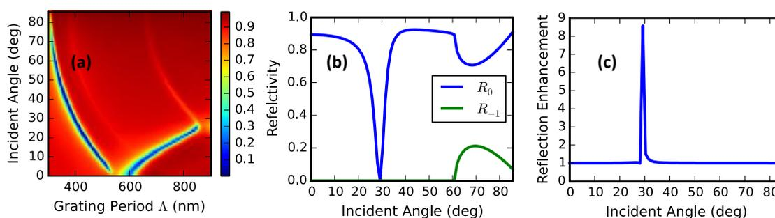
Fig. 2. (a) Grating reflectivity as a function of grating period  $\Lambda$  and incident angle  $\theta_i$  when illuminated by a TM plane wave at 750 nm. (b) 0 and -1 order diffraction with grating period  $\Lambda = 400$  nm. (c) 0 order reflectivity enhancement in a 400 nm grating illuminated by 750 nm wavelength when the MgO conductivity jumps from 0 to  $4.1 \times 10^7$  S/m. At resonant peak 29.95°, the reflection coefficient is enhanced 8.6 times.
